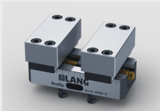
Thanks to threads in the base jaws, add-on jaws can also be mounted from the top for better accessibility towards the screws.
